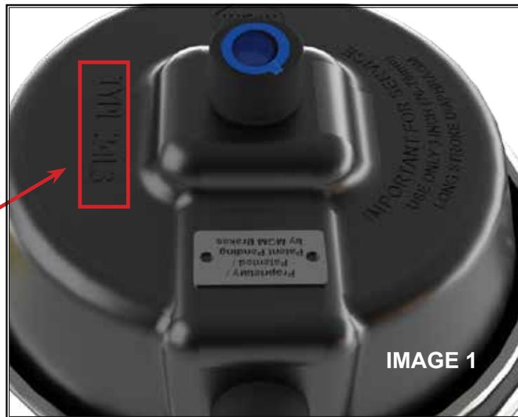
*Special note for type 20 and 24 long stroke chambers:* There are two sizes of these long stroke chambers. As shown in the long stroke clamp-type brake chamber data reference in the North American Standard Out-of-Service Criteria (OOSC), the rated stroke of these chambers could be 2.5 inches or 3 inches. Whenever the square embossment is 0.5 inch high, it indicates a long stroke chamber with a rated stroke of 3 inches, having a brake adjustment limit of 2.5 inches.
